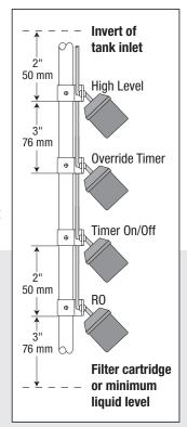
**NOTE:** If you use the general float settings, you may need to return at a later time and adjust float settings after the system is in operation.
