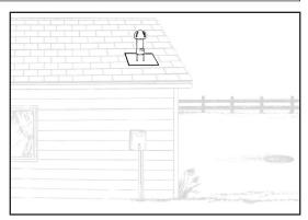
Carbon filters are often installed on roof vents to control odors. Use proper safety equipment and practices when working on roofs.
