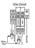
Use one wire nut to connect the pump and controls circuit breakers together with the incoming L1 power line. Use another wire nut to connect the pump and controls neutral blocks together with the incoming neutral line.
