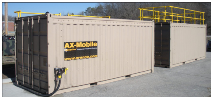
The NDCEE pilot project required custom AX-Mobile units that were built inside shipping containers.
