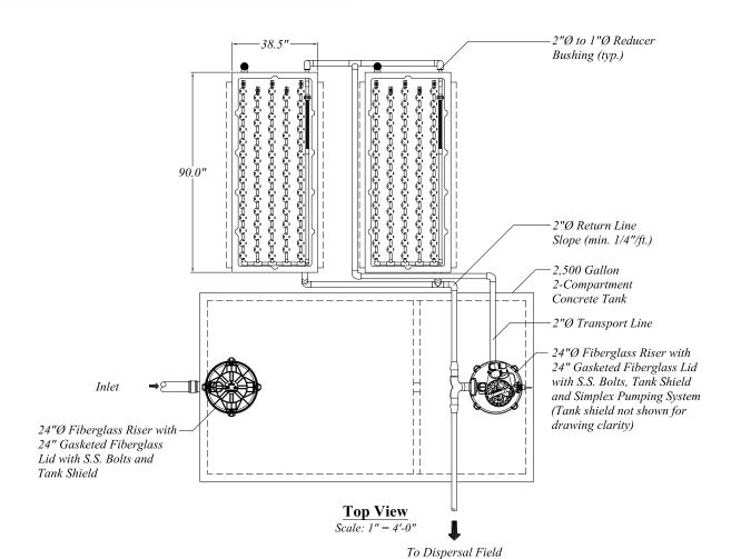
Processing Tank SizingBedroomsOccupants (maximum)2-Compartment Processing Tank (min. gallons)\*Single Compartment Septic Tank (min. gallons)5102,5001,5006123,0002,000
