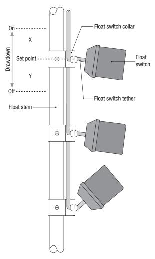
"On" and "Off" positions shown describe normally open float switches; "On" and "Off" positions are reversed for normally closed float switches
