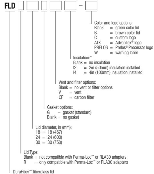
\* Insulation has an R-value of 10 per 2in (50mm) increment.
