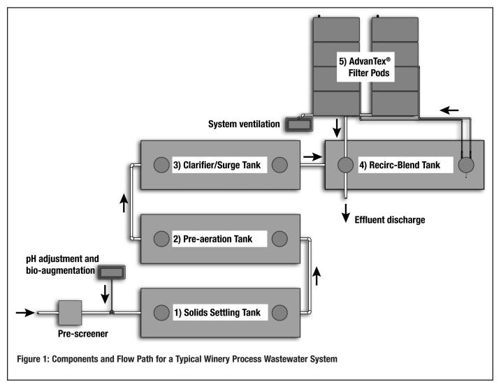
The primary tank should have three treatment compartments. Larger systems may use a tank for each compartment, instead.
