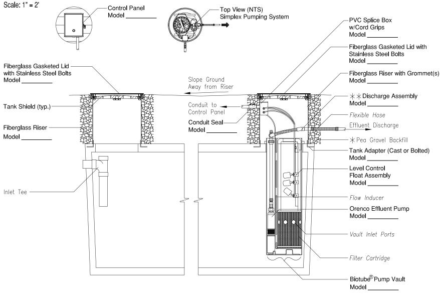
st Pea Gravel Backfill Recommended to Help Prevent Frost Heave
